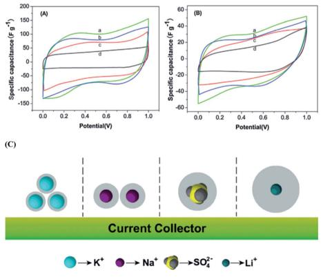
Fig. 10 CV curves of the supercapacitors with the electrolytes (2 M) (a) KOH, (b) NaOH, (c) LiOH and (d)  $Na_2SO_4$  at scan rates of (A) 5 mV s<sup>-1</sup> and (B) 100 mV s $^{-1}$ . (C) The ion of hydrated ionic radius on the MnFe<sub>2</sub>O<sub>4</sub>-based supercapacitors. This figure has been adapted from ref. 117 with permission from Elsevier.
