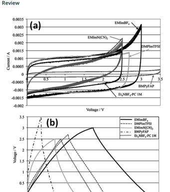
Fig. 18 (a) CV of various electrolytes at  $5 \text{ mV s}^{-1}$  and (b) galvanostatic charge–discharge at  $2 \text{ mA cm}^{-2}$ . This figure has been adapted from ref. 168 with permission from the Royal Society of Chemistry.
