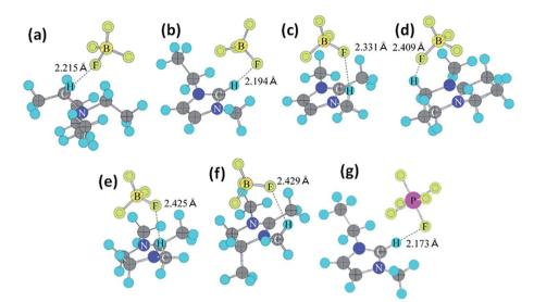
Fig. 15 Ion-pair structures in vacuo optimized using HF/6-31 + G(d,p), (a)  $TEA^+BF_4^-$ , (b)  $EMI^+BF_4^-$ , (c)  $TMI^+BF_4^-$ , (d)  $AMN^+BF_4^-$ , (e)  $TMIN^+BF_4^-$ , (f)  $TEMIN^+BF_4^-$ , and (g)  $EMI^+PF_6^-$ . This figure has been adapted from ref. 152 with permission from The Electrochemical Society.
