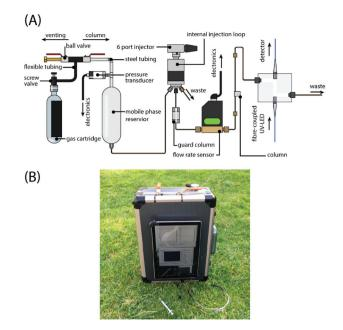
**Fig. 1** Portable high-performance liquid chromatography. (A) The schematic shows the key system components and their connectivity. The components are depicted for clarity and are not intended to dictate an orientation of operation. (B) Photograph of the 'chromatography in a suitcase' system running separations in the field.
