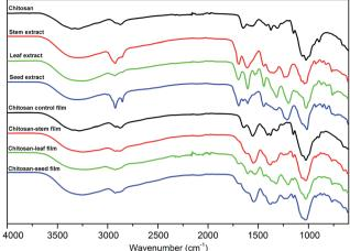
Fig. 1 FT-IR spectra of chitosan; stem, leaf and seed extracts of Pistacia terebinthus; chitosan control film; chitosan-stem film; chitosanleaf film and chitosan-seed film
