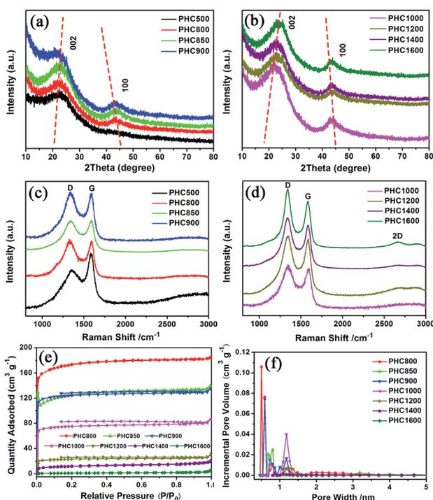
Fig. 2 Structure of PHC carbonized at different temperature. (a, b) XRD patterns; (c, d) Raman spectra; (e)  $\text{N}_2$  adsorption-desorption isotherms; (f) pore size distribution calculated by the BJH method.
