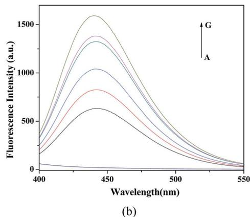
Fig. 8 (a) The reaction of TA with  $\cdot\text{OH}$ . (b) Fluorescent spectra of acetate buffer solution (pH = 4) containing only TA and PDI-CuO (A) or with H<sub>2</sub>O<sub>2</sub> (0.25 M), TA (0.5 mM) and the PDI-CuO nanocomposites with different concentration ((B) 0, (C) 20, (D) 80, (E) 200, (F) 250, (G) 300 μg mL $^{-1}$ ) were incubated at 55 °C for 30 min. The FL excitation wavelength was fixed at 315 nm.
