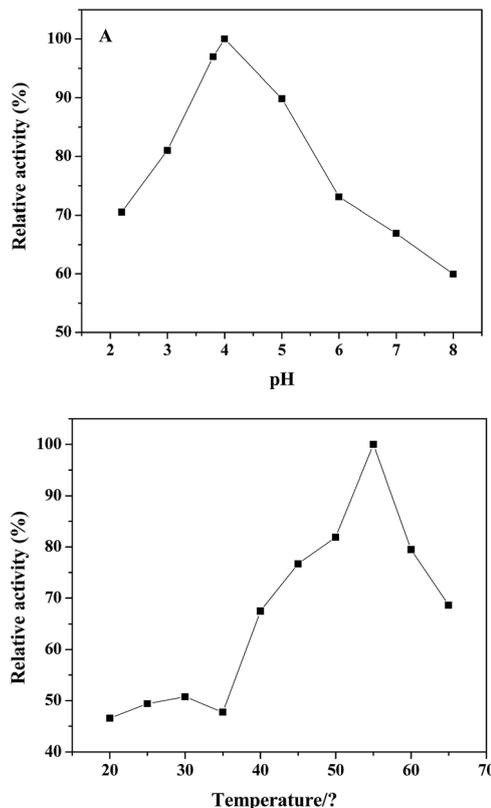
Fig. 6 The optimization of pH (A) and temperature (B) for the peroxidase-like activity of the PDI-CuO nanocomposites. Experiments were conducted by using 3 mg mL<sup>-1</sup> PDI-CuO in 2 mL of 1.4 mL buffer solution with 0.2 mL of 0.25 M H<sub>2</sub>O<sub>2</sub> and 0.2 mL of 2 mM TMB as substrates. In each curve, the relative activity was defined as the ratio of catalytic activity of the maximum catalytic activity.
