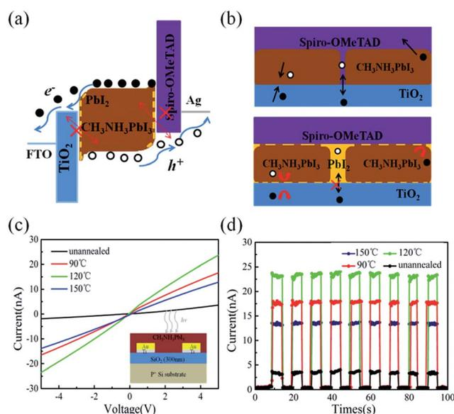
Fig. 7 Schematic diagram of (a) band gap of perovskite, PbI<sub>2</sub> and perovskite device after passivation, (b) electrons and holes transfer process in the pristine and passivated perovskite film. (c) The current–voltage ( $I$ - $V$ ) and (d) current–time ( $I$ - $t$ ) characteristic curves of the perovskite film annealed at different temperatures on the Si substrates under illumination (650 nm, 1 mW cm<sup>-2</sup>).
