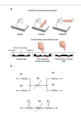
Fig. 2 Flexible microfluidic pressure sensor. (a) Working principle as a micropump system when the load is applied and removed, respectively. (b) Principle of operation illustrated using an electrical circuitry analogy
