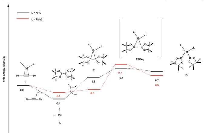
Fig. 2 Free energy profile (in kcal mol<sup>-1</sup>) for the oxidative addition pathways with bis-ligand complexes.
