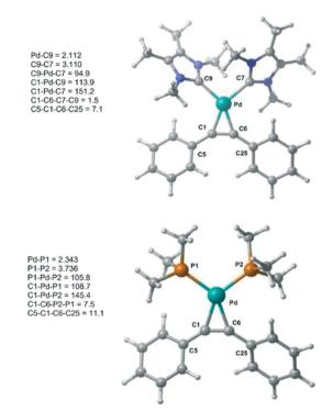
Fig. 1 Optimized structures of 1 and 1-PMe $_3$  at M06-L/BSI level of theory with selected bond lengths (Å) and angles (°).
