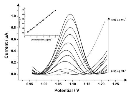
Fig. 3 Differential pulse voltammograms of the screen-printed graphite electrode by adding aliquots of PMA (in phosphate buffer pH 7.0) at concentrations in the range of  $0.50-4.98~\mu g~mL^{-1}$  (in phosphate buffer supporting electrolyte); the dotted line represents a blank. (inset) An analytical curve corresponding to the anodic peak for the oxidation of PMA over the concentration range (*E*-step: 0.002~V; *E*-pulse: 0.1~V; *t*-pulse: 0.05~V s<sup>-1</sup>; *t*-eq. 1 s).
