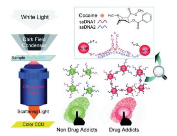
**Fig. 12** Principle of the nanoplasmonic imaging of latent fingermarks and the identification of cocaine in latent fingermarks by DFM. Peproduced from ref. 92 with permission from Wiley.
