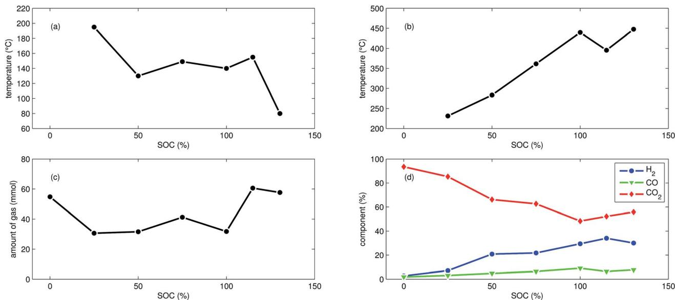
Fig. 5 Summary of all experiments with LFP cells at different SOC: (a) onset cell temperature  $\theta_o$ . (b) Maximum cell temperature  $\theta_m$ . (c) Amount of produced gas  $n_{sum}^{ideal}$ . (d) Main detected gas components  $r_i^{GC}$ .
