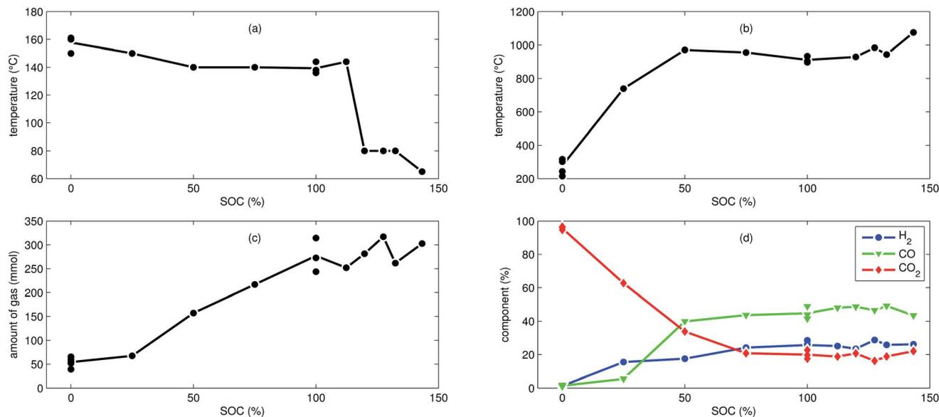
Fig. 3 Characteristic thermal runaway parameters from all NCA experiments. (a) Onset cell temperature  $\theta_o$ . (b) Maximum cell temperature  $\theta_m$ . (c) Amount of produced gas  $n_{sum}^{ideal}$ . (d) Main detected gas components  $r_i^{GC}$ .
