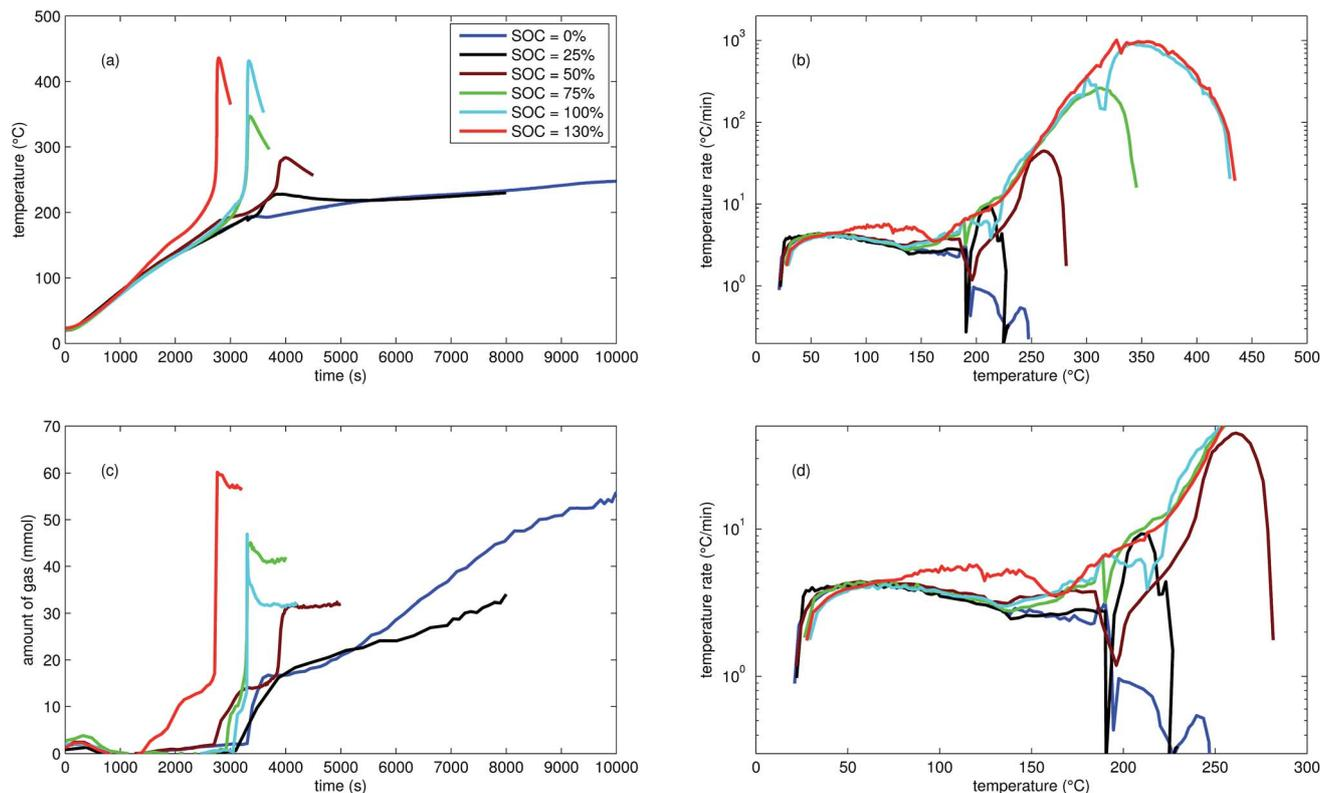
Fig. 4 Typical experiments with LFP cells: (a) cell temperature profiles. (c) Amount of produced vent-gas. (b) Cell temperature rate  $d\theta/dt$  vs. cell temperature  $\theta$ , full temperature range. (d) Close up view of the cell temperature rate.
