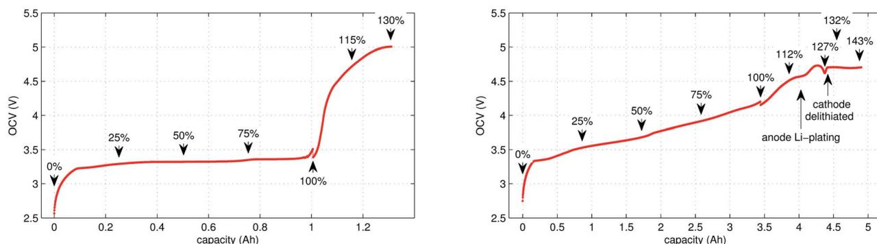
Fig. 1 OCV characteristics of the (left) LFP and (right) NCA cells. Measured values in the allowed voltage range and additionally in the overcharge region are given. SOC points, at which temperature-ramp experiments were done, are marked. Rough estimates, where Li-plating and complete cathode delithiation may occur, are indicated for the NCA cell. The discontinuities at 100% are caused by relaxations during the time-gaps between cycling and the overcharge experiments.
