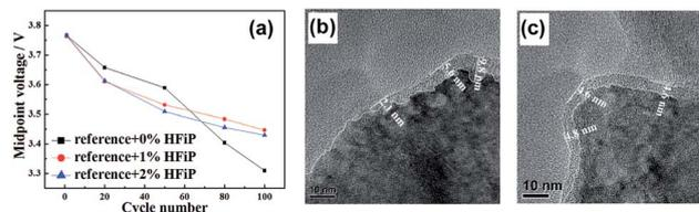
Fig. 24 Midpoint voltage of cells at a current density of 180 mA g<sup>-1</sup> in the voltage range of 2.0–4.6 V with electrolytes containing 0%, 1% and 2% HFIP additive. TEM images of Li[Li<sub>0.2</sub>Mn<sub>0.56</sub>Ni<sub>0.16</sub>Co<sub>0.08</sub>]O<sub>2</sub> cathodes in the electrolyte (b) without and (c) with HFIP additive at 18 mA g<sup>-1</sup> after 1 cycle. Reproduced with permission.<sup>115</sup>
