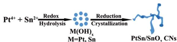
**Scheme 1** The growth mechanism of PtSn/SnO<sub>2</sub> CNs.
