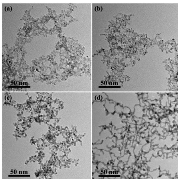
Fig. 4 TEM images of the products using  $\text{H}_2\text{PtCl}_6$  and  $\text{SnCl}_4$  (a),  $\text{K}_2\text{PtCl}_4$  and  $\text{SnCl}_4$  (b),  $\text{K}_2\text{PtCl}_4$  and  $\text{SnCl}_2$  (c) and  $\text{H}_2\text{PtCl}_6$  and  $\text{SnCl}_2$  (d) as metal precursors after 12 h reaction.
