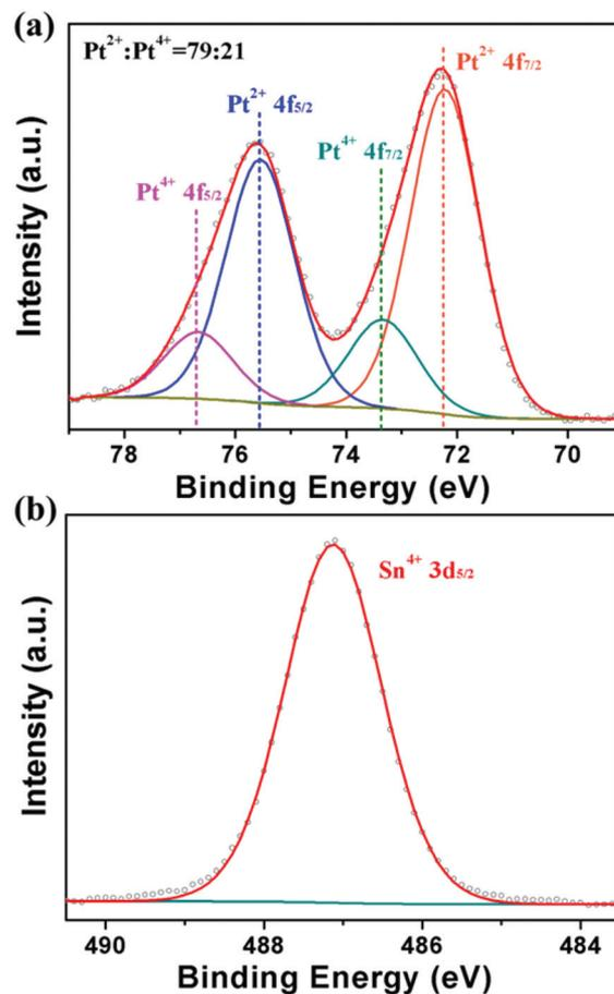
Fig. 3 XPS spectra of the as-obtained products for Pt 4f (a) and Sn 3d<sub>5/2</sub> (b) after mixing two metal precursors with stirring for 20 min.
