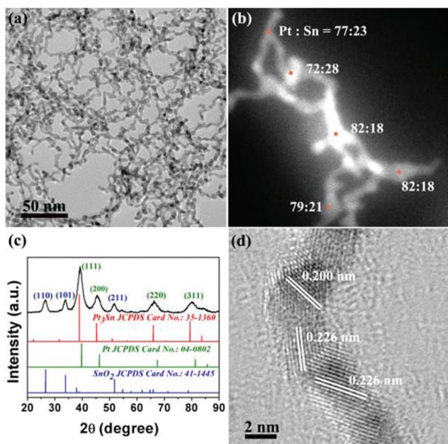
Fig. 1 TEM image (a), EDS spot scan image (b), PXRD pattern (c) and HRTEM image (d) of the as-obtained composites. For (c), marked lattice facets in dark blue belong to SnO<sub>2</sub>, green ones belong to Pt.
