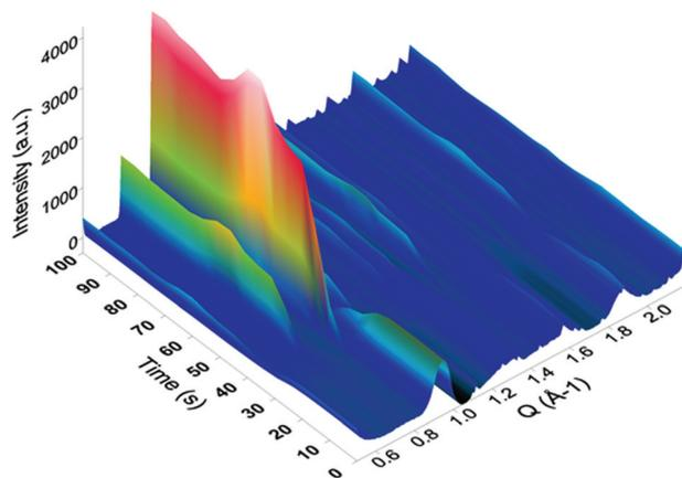
**Fig. 6** Nucleation and growth of HKUST-1\_2 at room temperature as a function of time when the alcoholic solution containing BTC is added to the solution containing Cu-based precursors\_2. The ligand was injected at  $t = 30$  seconds. A SAXS-based diffraction pattern of HKUST-1\_2 as a function of time shows that nucleation starts within 5 seconds after addition of the organic linkers.
