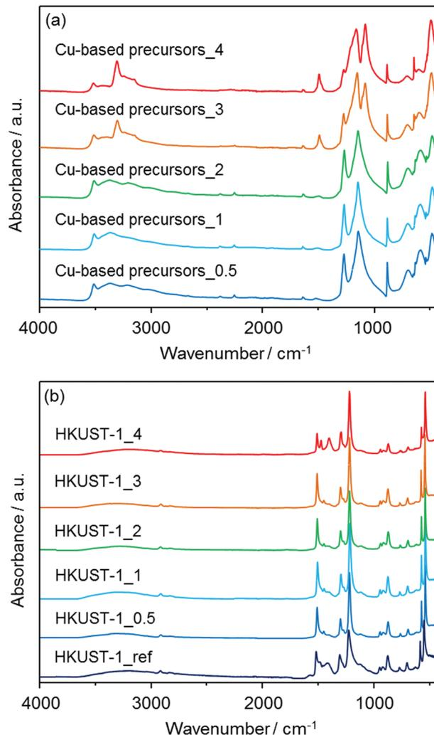
**Fig. 4** FT-IR spectra of (a) the solvent insoluble Cu-based precursors (Cu-based precursors<sub>X</sub>) and (b) corresponding HKUST-1<sub>X</sub> with HKUST-1<sub>ref</sub>.
