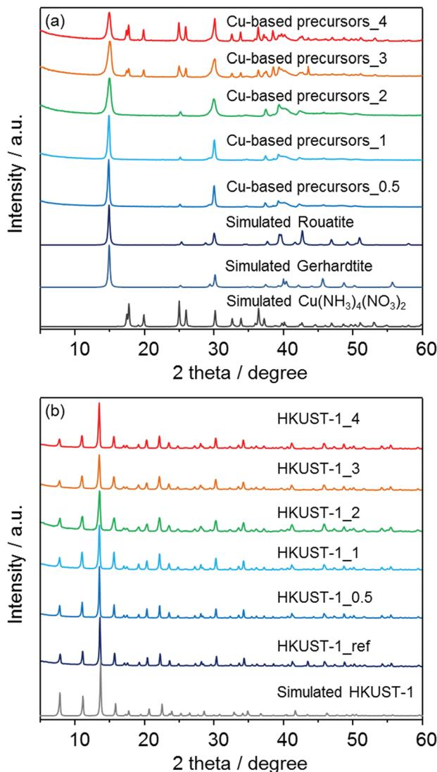
**Fig. 3** XRD patterns of (a) the solvent insoluble Cu-based precursors (Cu-based precursors<sub>X</sub>) with simulated patterns for  $\text{Cu}_2(\text{OH})_3\text{NO}_3$  (rouatite and gerhardtite) and  $\text{Cu}(\text{NH}_3)_4(\text{NO}_3)_2$  and (b) corresponding HKUST-1<sub>X</sub> with HKUST-1<sub>ref</sub> and simulated pattern for HKUST-1.
