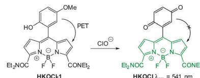
Fig. 86 Structure and reaction of HKOCl-1 with \text{ClO}^- .
