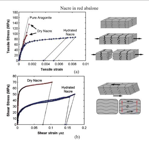
Fig. 14 (a) Tensile and (b) shear stress-strain curves for nacre in red abalone and a schematic of lamellar tile structures showing associated deformation modes. Tablet waviness generates resistance to sliding, accompanied by lateral expansion (vertical arrows). 48,104
