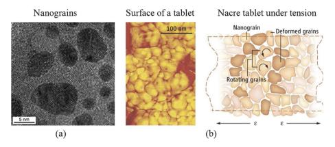
Fig. 8 (a) High-resolution TEM (face-on view) of a tablet from the nacreous layer of a red abalone specimen showing nanograins of about 3–10 nm in size;<sup>31</sup> (b) (left) AFM image of surface nanograins on an individual nacre platelet from California red abalone and (right) schematic of nanograin rotation under tension.<sup>38,39</sup>
