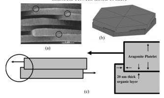
**Fig. 11** (a) SEM image of nacre from red abalone showing the presence of interlocks, indicated by circles; (b) schematic illustration showing interlocks between platelets of nacre, showing that rotation of layers of platelets is essential for the formation of platelet interlocks. (c) Schematic illustration showing the mechanism of loading through a cross-section cut across platelets and through the interlocks. <sup>41</sup>
