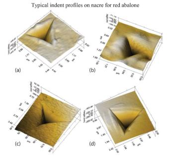
**Fig. 17** Typical indent profiles on nacre from red abalone: (a) dry nacre, there are pile-ups around the edges; (b) wet nacre, the blunted appearance of the indentation is related to the compliance of the wet nacre seen from its relatively low modulus; (c) heat treated nacre, the material appears compacted and similar to what happens to sand when it is heated and grains begin to fuse together; and (d) monolithic aragonite, the uneven pile-up indicates anisotropy. <sup>109</sup>
