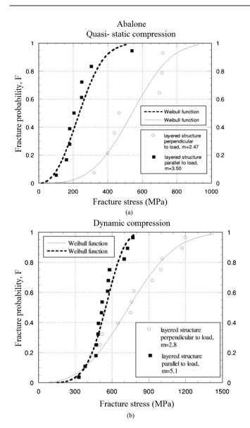
Fig. 16 Weibull plots of abalone nacre in abalone under (a) quasi-static, and (b) dynamic compressive loading.  $^{46}$
