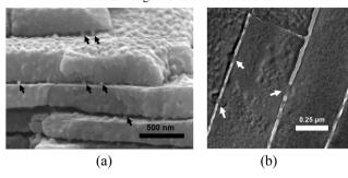
**Fig. 5** TEM images of the red abalone nacre cross-section showing (a) mineral bridges between tile interfaces and (b) mineral bridges between tablets of neighboring layers shown by arrows. <sup>79</sup> These mineral bridges are also found in bivalves.
