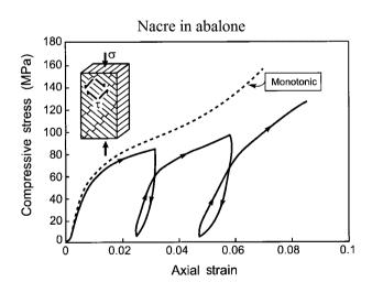
**Fig. 15** Compression stress–strain curves for nacre in abalone, representing interlamellar shear, measured both in monotonic loading and with loading–unloading loops. The insert indicates that the lamellae boundaries are orientated at 45° to the loading axis.<sup>5</sup>
