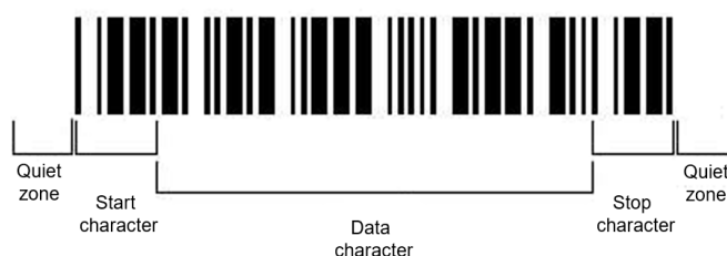
Fig. 2 Schematic view of a 1D code.
