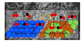
Sodium cobaltate works as a bifunctional material, in the catalysis of CO oxidation and subsequent  $CO_2$  chemisorption.
