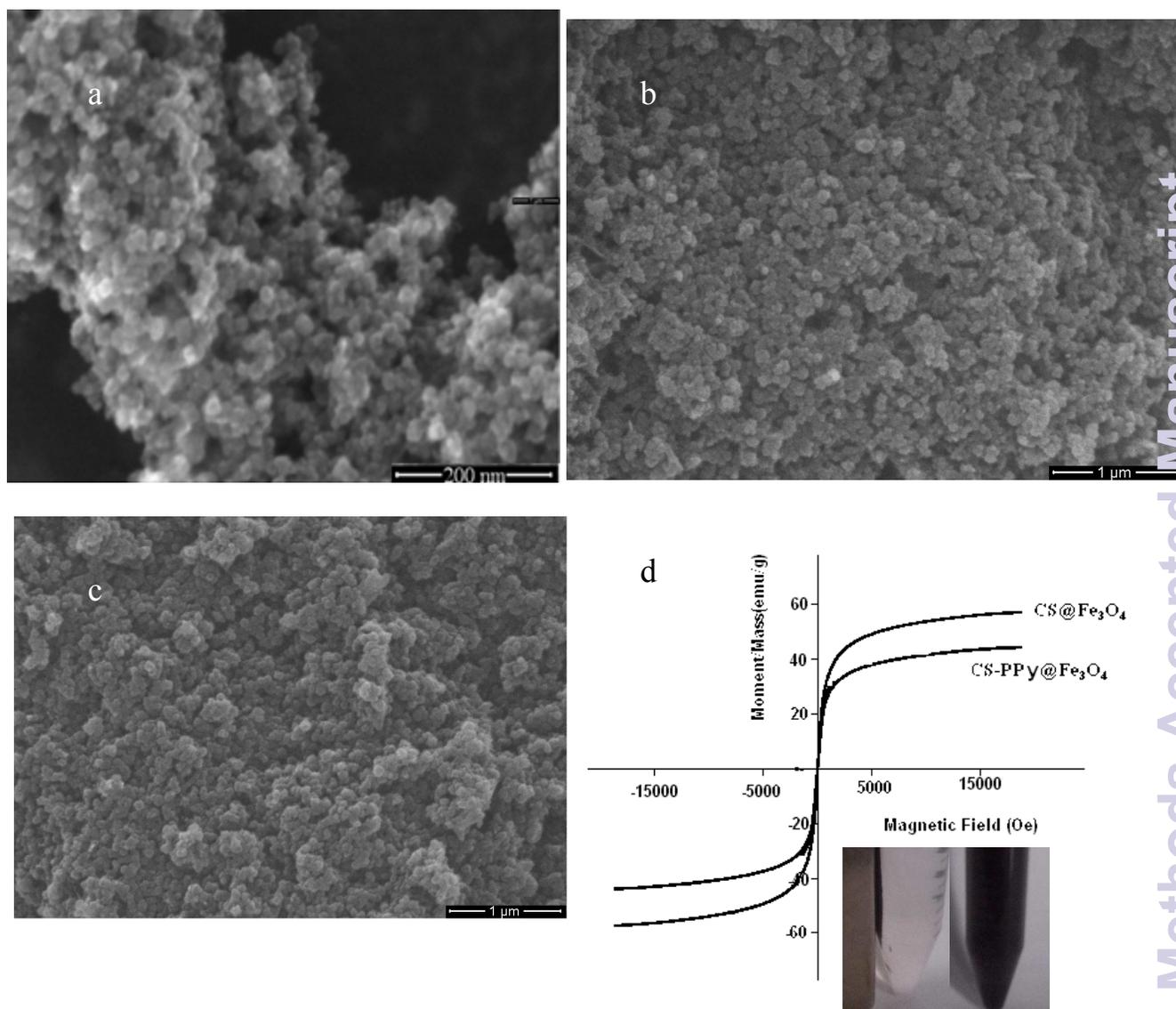
**Fig. 2** (a) SEM images of Fe<sub>3</sub>O<sub>4</sub>; (b) CS@Fe<sub>3</sub>O<sub>4</sub>; (c) CS-PPy@Fe<sub>3</sub>O<sub>4</sub>; (d) magnetic curves of CS@Fe<sub>3</sub>O<sub>4</sub> and CS-PPy@Fe<sub>3</sub>O<sub>4</sub>. The inset shows the separation-redispersion process of CS-PPy@Fe<sub>3</sub>O<sub>4</sub>.
