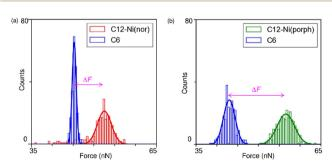
**Fig. 3** Histograms of the observed adhesive force constructed from the 256 force curves for (a) the C6 matrix with and without C12–Ni(nor) and (b) the C6 matrix with and without C12–Ni(porph). The bold lines are the result of the Gaussian fitting of the histograms.  $\Delta F$  is the difference between peak adhesion forces for C6 and C12–Ni(nor) or C6 and C12–Ni(porph).
