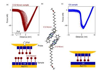
Fig. 2 (a) and (c) Force curves measured on the C6 matrix with and without C12–Ni(nor). Adhesion force was defined as the maximum attraction (most negative force signal value) measured by the force curve. Schematics of the experimental systems are shown at the bottom. (b) Schematic illustration of the  $\pi$ -stack formation between C12–Ni(nor) molecules. Grey, white, blue, red, yellow, and green balls correspond to C, H, N, O, S and Ni atoms, respectively.
