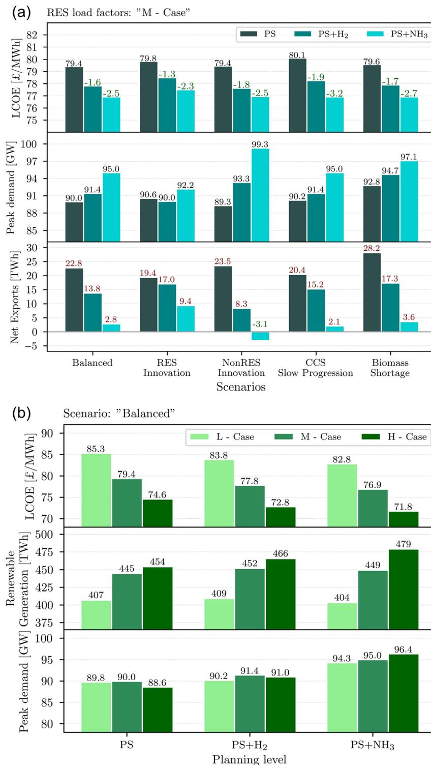
Fig. 14 Scenario analysis for the case study of GB in 2040 over: (a) various build rate scenarios and the planning levels and (b) the planning levels and RES load factors for "Balanced" scenario.
