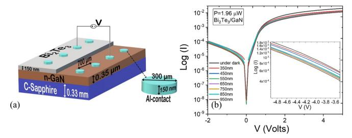
Fig. 1 (a) Schematic of the device structure of Bi<sub>2</sub>Te<sub>3</sub>/n-GaN/S. (b) Plot of the semi-log (I-V) characteristics for the Bi<sub>2</sub>Te<sub>3</sub>/n-GaN heterojunction device under dark and illumination conditions when the wavelength of the irradiating wavelength of the light was varied from 350 nm to 950 nm at a constant incident light power of 1.96  $\mu$ W; inset shows the reverse saturation current in the reverse bias (V) = -4.8 V to -3.6 V.
