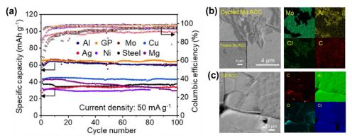
Fig. 10 Electrochemical measurements and ex situ characterization of different anodic CCs. (a) Cycling performance of different anodic CCs at a fixed rate of 50 mA  $g^{-1}$  (b) SEM and EDX measurements of fully discharged Mo anodic CC after 100 cycles. (c) AES image and corresponding AES elemental mapping of fully charged GP anodic CC etched for 20 min by argon ion bombardment. Reprinted with permission, <sup>128</sup> Elsevier, Copyright 2022.
