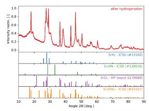
Fig. 10 XRD patterns of the solid product of Sr<sub>2</sub>N-hydrogenation (see Fig. 7). Peak intensities have been normalized.
