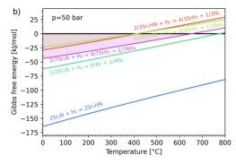
Fig. 4 Ellingham diagram of the hydrogenation step for the reactions (7)–(11). Variation of the Gibbs free energy change per mol  $H_2$  as a function of temperature for: (a) standard  $\Delta G_{\rm rxn}^{\circ}$ ; and (b)  $\Delta G_{\rm rxn}$  at 50 bar assuming 20% reaction extent.
