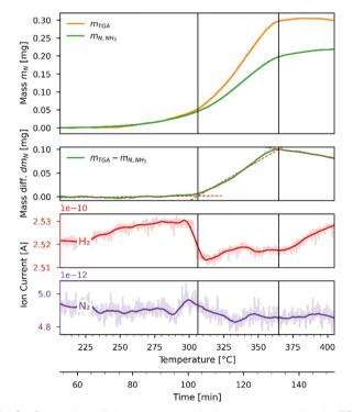
Fig. 8 Comparison of nitrogen mass equivalents as measured by the TGA (orange) and the NH3 analyzer (green) as a function of time and temperature during the Sr<sub>2</sub>N-hydrogenation run of Fig. 7. The top plot shows the measured and predicted nitrogen masses in mg. The second plot shows the difference between the TGA and NH<sub>3</sub> analyzer nitrogen mass in mg. The bottom plots show the ion current (recorded by the mass spectrometer) for H2 (red) and N2 (purple).
