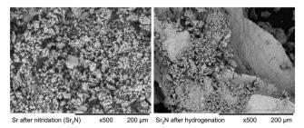
Fig. 11 SEM images of the solid products of Sr-nitridation (left) and Sr<sub>2</sub>Nhydrogenation (right) (500× magnification).
