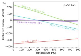
Fig. 3 Ellingham diagram of the nitridation step for reactions (3)–(6). Variation of the Gibbs free energy change per mol  $N_2$  as a function of temperature for (a) standard  $\Delta G_{\text{rxn}}^{\circ}$ ; and (b)  $\Delta G_{\text{rxn}}$  at 50 bar assuming 20% reaction extent.
