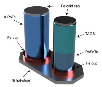
Fig. 6 Illustration of thermoelectric (TE) unicouple used in the multimission radioisotope thermoelectric generator (MMRTG), featuring n-type PbTe and a segmented p-type leg design. In the segmented p-type leg, PbSbTe is positioned near the hot side, while (GeTe)<sub>100-x</sub>(AgSbTe<sub>2</sub>)<sub>x</sub>, known as TAGS, is placed closer to the cold side. This rendering was created by the authors based on the original figure<sup>3</sup> (Image credit: NASA/ JPL/Caltech).
