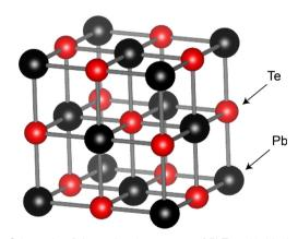
Fig. 8 Schematic of the rock-salt structure of PbTe, with black and red spheres representing Pb and Te atoms, respectively. The crystal structure information was retrieved from the Materials Project database and visualized using the VESTA software.48
