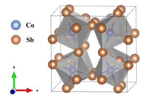
Fig. 11 Illustration of the crystal structure of the  $CoSb_3$ -based alloy, which crystallizes into octahedrons within the space group  $Im\overline{3}$ . The structure is characterized by a void at the center of the cubic lattice. Crystal structure information was sourced from materialproject.org and visually represented using VESTA.<sup>48</sup>
