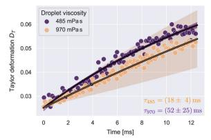
Fig. 3 Taylor deformation vs. time for silicone oil droplets at the stable extension rate. The solid lines illustrate fit curves of eqn (29) to the datapoints. Shaded regions show the  $2-\sigma$  error band of the fit data. The number of droplets N per condition was:  $N_{485} = 90$ ,  $N_{970} = 421$ .
