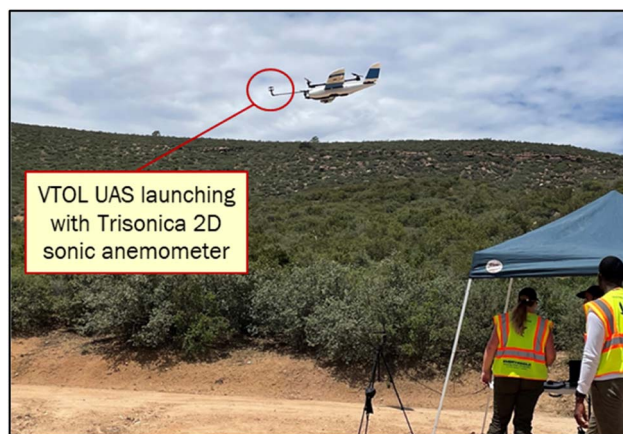
Fig. 18 Instrumented VTOL fixed-wing aircraft launching in airspace with 3 multirotors airborne nearby. The multirotors are not shown in this figure but are flying concurrent vertical profiles illustrated in Fig. 20 and 21.
