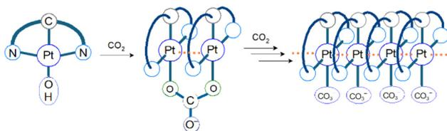
**Fig. 2** An image of aggregation resulting from the reaction of complex **1** with  $\text{CO}_2$  in basic aqueous solution. The  $\text{CO}_2$  gas bubbling causes the aggregate formation. The degree of aggregation increases up to at least 32.
