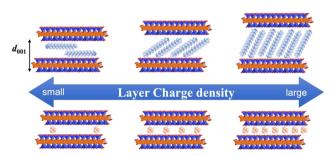
Fig. 25 Schematic of the variation in the arrangements of the intercalated alkylammonium ions in 2:1-type phyllosilicates depending on layer charge density
