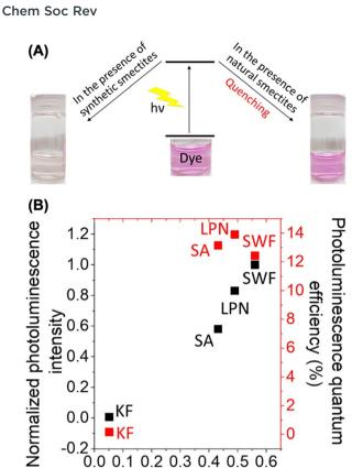
Fig. 19 (A) Photograph of an organic luminophore (Rhodamine 6G) and (B) relationship of the photodecolorisation rate constant with the normalised photoluminescence intensity (black) and the photoluminescence quantum efficiency (red) of SWF-R6G, SA-R6G, LPN-R6G, and KF-R6G suspensions.396
