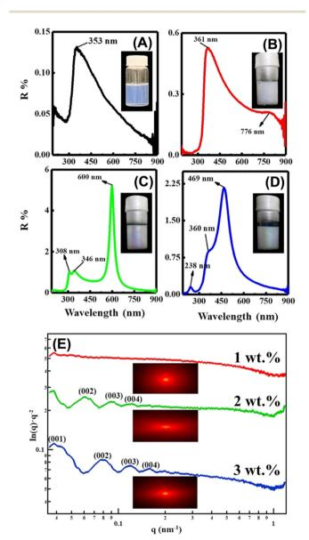
Fig. 36 Structural color of the liquid crystalline perovskite nanosheet suspension. (A)-(D) UV-Vis reflectance spectra and photographs of the colloids with the nanosheet concentration of (A) 0.1, (B) 1, (C) 2 and (D) 3 wt%. (E) Small-angle X-ray scattering and 2D patterns of the colloids with 1, 2 and 3 wt% of nanosheets. Reprinted from ref. 597. Copyright (2021), John Wilev & Sons
