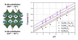
Fig. 33 Controlling the flat band position of perovskite nanosheet by isomorphous substitution of A or B site. The flat band potential of the nanosheets with varied compositions on a tin oxide-coated glass was measured by Mott-Schottky method under valid pH. 573 The measured values are in good agreement with the Fermi level values estimated based on Matsumoto's empirical correlation between the conduction band-edge positions and band gap energies for metal oxide semiconductors (solid lines). 572
