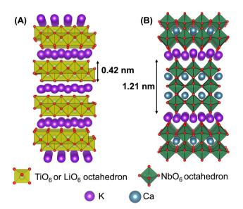
Fig. 30 Crystal structures of (A) lepidocrocite-type layered titanate  $K_{0.8} Ti_{1.73} Li_{0.27} O_4$  and (B) Dion–Jacobson-type layered perovskite  $KCa_2 Nb_3 O_{10}$ . The structural parameters were referred from ref. 528 and 529, respectively. The crystal structure was drawn using the VESTA program.  $^{44}$
