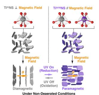
**Fig. 28** Schematics of the magnetic orientation,  $Ti^{4+}$ -based nanosheet ( $Ti^{IV}NS$ ; left) and its reduced form containing  $Ti^{3+}$  species ( $Ti^{IV/III}NS$ ; right) orient their 2D planes orthogonal and parallel to the applied magnetic field, respectively. Reprinted from ref. 507. Copyright (2018), the American Chemical Society.
