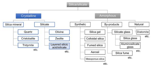
Fig. 8 Classification of crystalline and amorphous silica/silicates.
