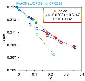
Fig. 6 Relationships between the lattice parameter a and composition x in the reported MgGa-LDHs. Diamonds are for iodide-type MgGa-LDHs<sup>130</sup> and circles are for the carbonate-type MgGa-LDHs. 131-134
