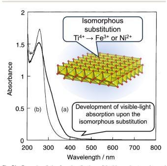
Fig. 31 Example of the functionalisation of lepidocrocite-type layered titanate by isomorphous substitution; development of visible-light absorption and red-shift in the light absorption edge. The absorption spectra correspond to an aqueous colloidal suspension (0.16 g dm<sup>-3</sup>) of nanosheets derived from the protonated forms of (a) K<sub>0.8</sub>Ti<sub>1.2</sub>Fe<sub>0.8</sub>O<sub>4</sub> and (b)  $K_{0.8}Ti_{1.6}Ni_{0.4}O_4$ . 566
