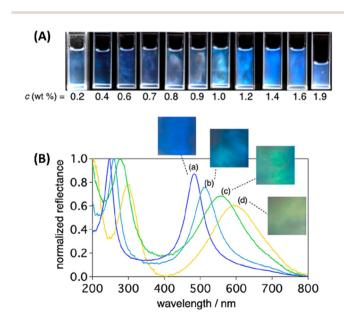
Fig. 15 (A) Photographs of nanosheet colloids (average nanosheet diameter of 1.8 μm) with various nanosheet concentrations c. (B) Photographs and UV-Vis spectra of the nanosheet colloid with the average nanosheet diameter of (a) 0.14, (b) 0.16 (c) 0.98, and (d) 1.8  $\mu m$ . The spectra were recorded at an observing angle of 10°.302
