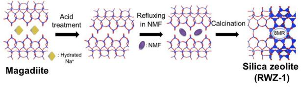
Fig. 11 Schematic of the topotactic conversion of magadiite into a silica zeolite (RWZ-1) during refluxing in N-methylformamide (NMF) and subsequent calcination. Reprinted from ref. 251 with permission from John Wiley & Sons
