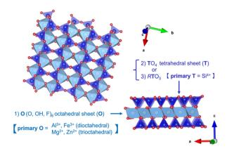
Fig. 14 Structure of a 2:1-type phyllosilicate, two TO<sub>4</sub> (the primary element of  $T = Si^{4+}$ ) tetrahedral sheets (T) on each side of an O (O, OH, F) octahedral sheet (O) occupied by octahedrally coordinated cations (e.g., Mg<sup>2+</sup>, Zn<sup>2+</sup>/Al<sup>3+</sup>, Fe<sup>3+</sup>, etc.), forming a T-O-T layer (prepared using VESTA software).44
