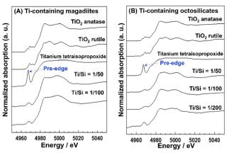
Fig. 9 (A) XANES spectra of the Ti-containing magadiites and reference (B) XANES spectra of the Ti-containing octosilicates and ref. 245.
