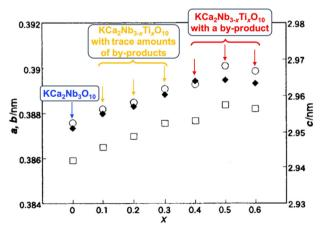
Fig. 35 Variation in the lattice parameters of  $KCa_2Nb_{3-x}Ti_xO_{10}$  by isomorphous substitution, where an increase in the lattice parameters of  $KCa_2Nb_{3-x}Ti_xO_{10}$  are correlated with x, according to Vegard's law. 554
