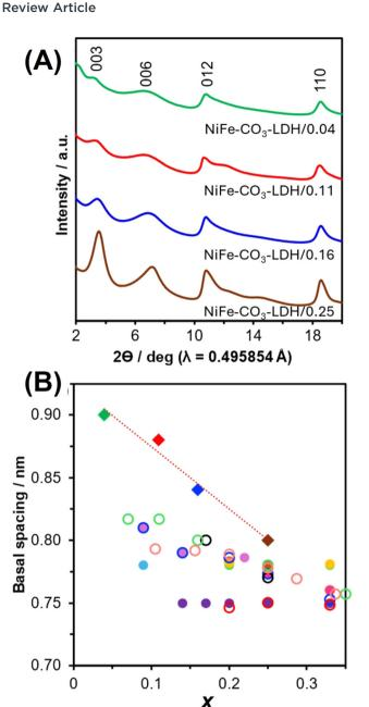
Fig. 7 (A) XRD patterns of NiFe-CO<sub>3</sub>-LDH/x, where x is 0.04, 0.11, 0.16, and 0.25. (B) Relationship between the basal spacing and x. Diamonds are values for NiFe-CO<sub>3</sub>-LDH/x, 134 closed circles are values reported for NiFe-CO<sub>3</sub>-LDHs, <sup>135-140</sup> and open circles are values reported for MgAl-CO<sub>3</sub>-LDHs, <sup>118,141</sup> MgGa-CO<sub>3</sub>-LDHs, <sup>133</sup> MgFe-CO<sub>3</sub>-LDHs, <sup>142</sup> and NiAl-CO<sub>3</sub>-LDHs.<sup>143</sup>
