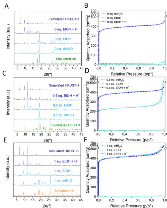
Fig. 1 XRPD patterns (left) and N<sub>2</sub> sorption isotherms (right) of Cu-BTC materials synthesized with (A, B) 0 equivalents, (C, D) 0.5 equivalents and (E, F) 1 equivalent of HCl and the corresponding products washed with water (ddH<sub>2</sub>O), ethanol (EtOH) or ethanol and acid (EtOH + H<sup>+</sup>). H0: CCDC 609754,<sup>11</sup> H1: CCDC 1288676.<sup>12</sup>
