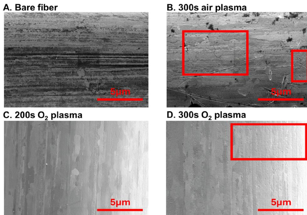
**Fig. 2** SEM images of gold fibers before and after treatment. (A) An example of an untreated gold fiber. (B) A representative example of a gold fiber treated with air plasma. Surface pitting is visible. (C) An example image of a fiber treated with oxygen plasma for 200 s. (D) An example image of a fiber treated with 300 s of oxygen plasma showing pitting. Scale bars are shown on each image. Red box highlights the noted pitting observed.
