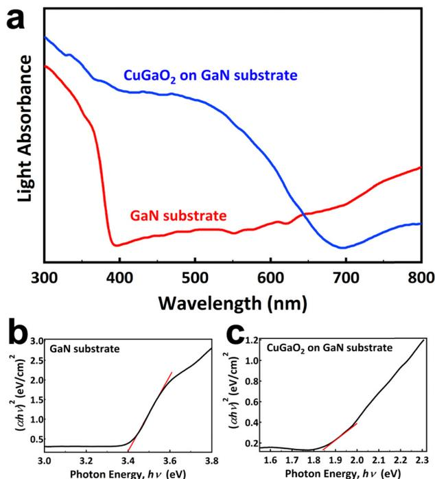
Fig. 4 (a) UV-Vis diffused reflectance spectra of the GaN substrate and CuGa<sub>2</sub>O<sub>4</sub> on GaN, and bandgap estimation of (b) the GaN substrate and (c) CuGa<sub>2</sub>O<sub>4</sub> on GaN samples.
