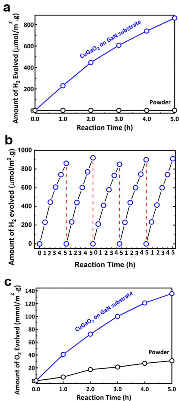
Fig. 5 (a) Photocatalytic hydrogen generation of powder and CuGa<sub>2</sub>O<sub>4</sub> on GaN samples, (b) three cycles for the stability test of hydrogen generation of the CuGa<sub>2</sub>O<sub>4</sub> on GaN sample, and (c) photocatalytic oxygen generation of powder and CuGa<sub>2</sub>O<sub>4</sub> on GaN samples.
