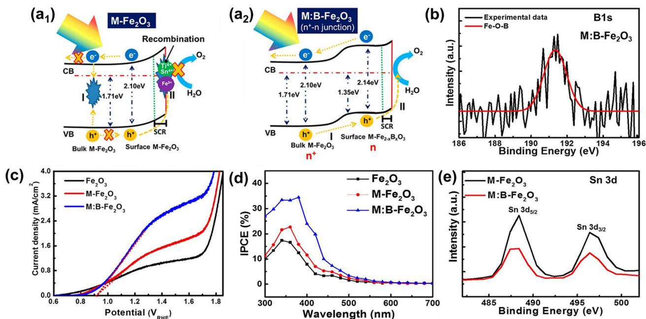
Fig. 10 (a) Schematic illustration of an energy band diagram and charge transfer process of (a<sub>1</sub>) M-Fe<sub>2</sub>O<sub>3</sub> and (a<sub>2</sub>) M:B-Fe<sub>2</sub>O<sub>3</sub>, (b) XPS B 1s spectra, (c) *J*-*V* curves, (d) IPCE, and (e) XPS Sn 3d spectra. Reproduced from ref. 44 with permission from American Chemical Society, Copyright 2018.
