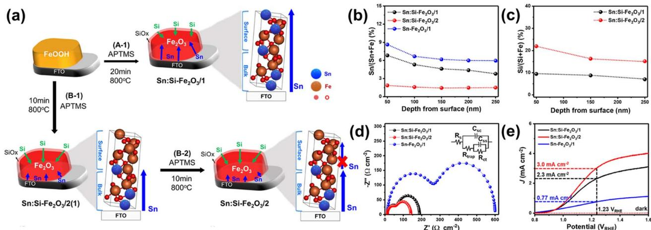
Fig. 12 (a) Fabrication procedures of Sn:Si-Fe<sub>2</sub>O<sub>3</sub>/1 and Sn:Si-Fe<sub>2</sub>O<sub>3</sub>/2. (b) XPS depth profiles of Si and (c) Sn according to the depth from the surface of Sn:Si-Fe<sub>2</sub>O<sub>3</sub>/1–2. (d) EIS measurements at 1.23 V<sub>RHE</sub>, and (e) *J–V* curves of Sn:Si-Fe<sub>2</sub>O<sub>3</sub>/1–2, and Sn-Fe<sub>2</sub>O<sub>3</sub>/1. Reproduced from ref. 65 with permission from American Chemical Society, Copyright 2021.
