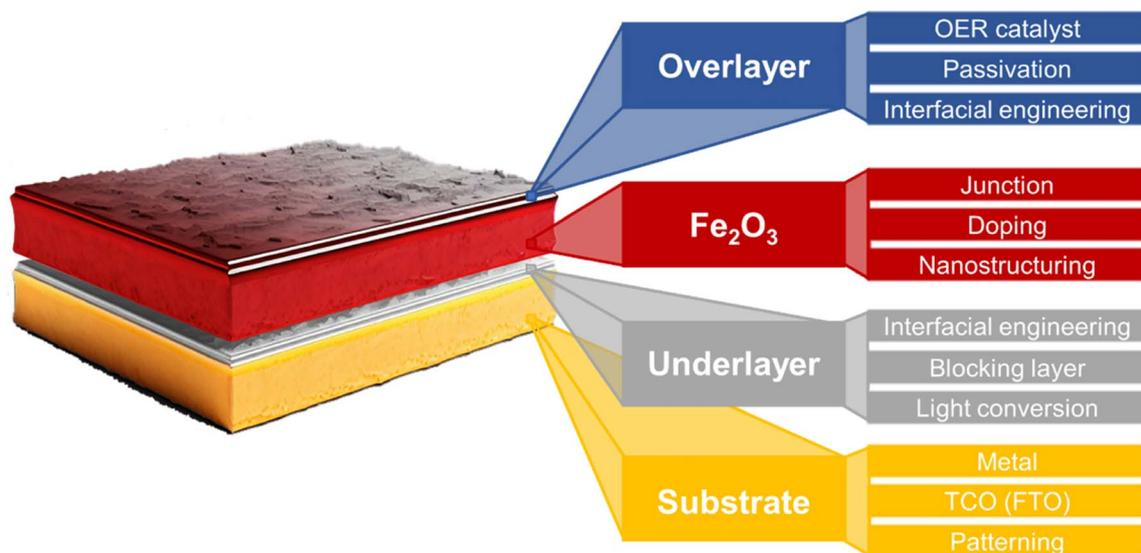
Fig. 3 Schematic illustration of various strategies for enhancing PEC efficiencies of a hematite photoanode.<sup>35–43</sup>
