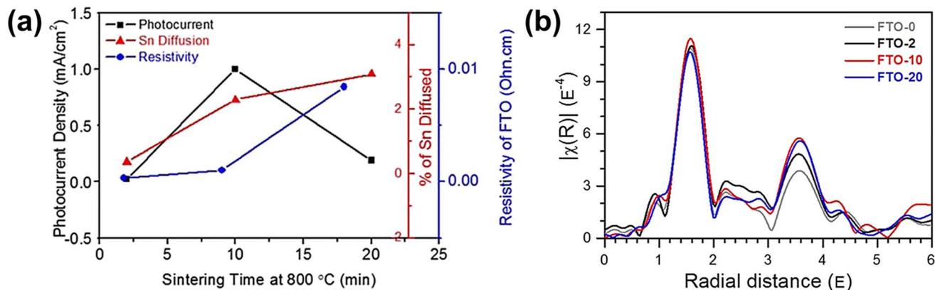
Fig. 8 (a) Photocurrent density (mA cm<sup>-2</sup>), atomic percent of Sn diffusion of hematite photoanodes, and resistivity of the FTO substrate sintered at 800 °C for 2, 10, and 20 min.  $k^3$ -weighted Fourier transforms for (b) Sn K-edge EXAFS of FTO substrates sintered at 800 °C for 0, 2, 10, and 20 min. Reproduced from ref. 62 with permission from American Chemical Society, Copyright 2015.
