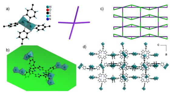
Fig. 8 Crystal structure of CatPMOF-2(Al). (a) Inorganic SBU (left) acting as a distorted square planar node (right); (b)  $H_2$ TcatPP ligand, with the mean plane of the macrocycle shown in green; (c) **cds** net (the ligand and the inorganic SBU are shown in green and violet, respectively); (d) full structure shown along the b axis.
