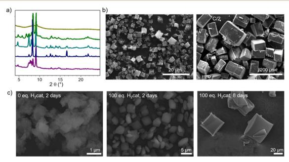
Fig. 3 (a) PXRD patterns of the samples synthesized in various solvents; from top to down: pure DEF, DEF/ $H_2O = 3$ , DEF/ $H_2O = 1$ , and DEF/ $H_2O = 1$ . = 1 and concentration lowered twice, DEF/H<sub>2</sub>O = 1/3; (b) SEM images of CatPMOF-2(Al): effect of the concentration of reactants; (c) SEM images of Ni-CatPMOF-2(Al): effect of the amount of  $H_2$ cat and reaction time ( $H_{10}$ TcatPP/AlCl<sub>3</sub> = 1/2, DEF, and 160 °C).
