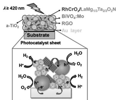
Fig. 5 Schematic of a-TiO 2 -coated (RhCrO x /ZrO 2 /LaMg 1/3 Ta 2/3 O 2 N)/(Au, RGO)/BiVO 4 :Mo photocatalyst sheet. Adapted with permission from ref. 44. Copyright 2016 Wiley-VCH.
