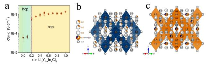
Fig. 6 (a) Ionic conductivity of  $\text{Li}_3 Y_{1-x} \text{In}_x \text{Cl}_6$  with different In contents at 25 °C. Reproduced with permission.<sup>38</sup> Copyright 2020, American Chemical Society. Structure (b) and the main 3D Li ion diffusion pathway (c) of  $\text{Li}_2 \text{In}_{1/3} \text{Sc}_{1/3} \text{Cl}_4$ . Reproduced with permission.<sup>46</sup> Copyright 2022, Springer Nature.
