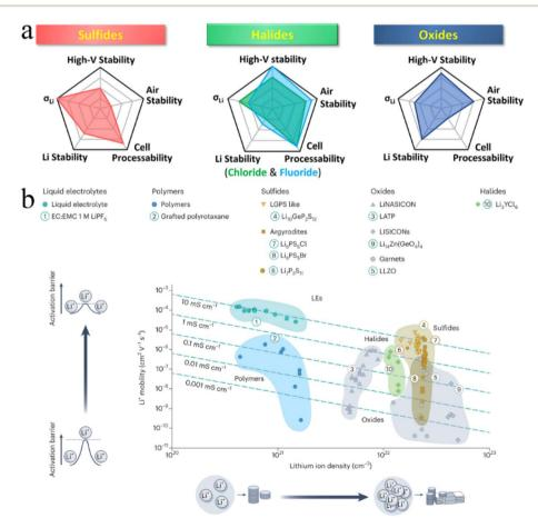
Fig. 1 (a) Spider plots exhibiting various properties of three typical inorganic SSEs. Reproduced with permission.<sup>19</sup> Copyright 2022, American Chemical Society. (b) Comparison of the ionic conductivity of different electrolytes based on the Li content. Reproduced with permission.<sup>18</sup> Copyright 2023, Springer Nature.
