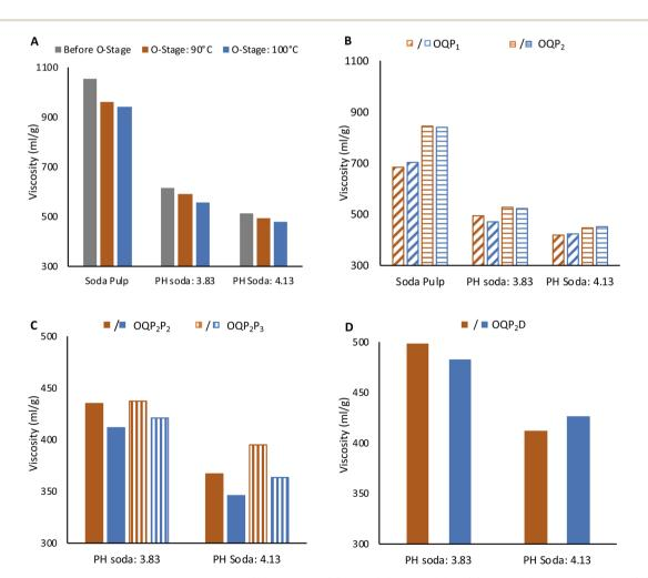
Fig. 3 CUEN viscosity of pulps before and after oxygen (O) bleaching (A) after OQP<sub>1</sub> and OQP<sub>2</sub> (B), after OQP<sub>2</sub>P<sub>2</sub> and OQP<sub>2</sub>P<sub>3</sub> (C) and after OQP<sub>2</sub>D (D) (temperature of O-stage in the sequences are indicated by for 90 °C and for 100 °C).
