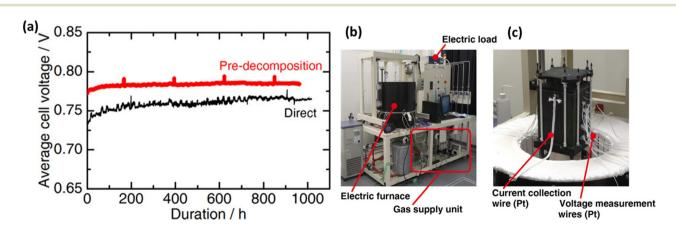
Fig. 9 (a) Average cell voltage during a 1000 h durability test with ammonia fuel at 700 °C, 0.316 A cm<sup>-2</sup> current density, the photograph of (b) the stack evaluation system and (c) the 30-cell SOFC stack. Reproduced with permission.<sup>58</sup> Copyright 2020, Wiley-VCH.
