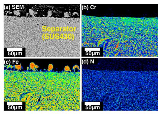
Fig. 10 Cross-sectional images of the separator on the anode side after a 1000 h durability test with direct ammonia fuel at 700 °C, 0.316 A cm<sup>-2</sup> current density: (a) scanning electron microscopy image, and the distribution of (b) Cr, (c) Fe, and (d) N. Reproduced with permission.<sup>58</sup> Copyright 2020, Wiley-VCH.
