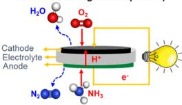
Fig. 4 Schematic representation of a direct ammonia solid oxide fuel cell based on oxide-ion-conducting (O-DASOFC) and proton-conducting (H-DASOFC) electrolytes.
