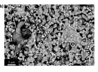
Fig. 5 (a) XRD pattern of Ni film on a YSZ disk after exposure to ammonia (100 mL min<sup>-1</sup>) at 600 °C for 1 h. Reproduced with permission.<sup>36</sup> Copyright 2015, American Chemical Society. (b) SEM image of the anode surface at the fuel inlet region. Reproduced with permission. <sup>56</sup> Copyright 2019, Elsevier.
