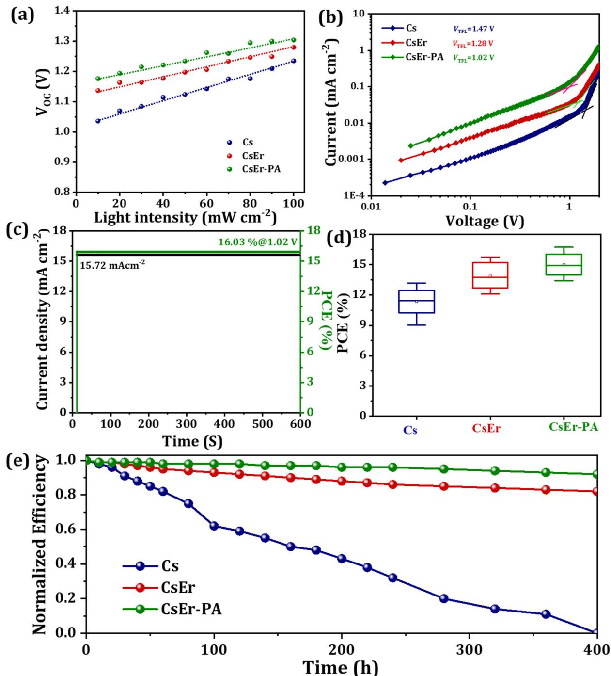
**Fig. 5** (a)  $V_{oc}$  as a function of light intensity, (b) dark current–voltage curves of electron-only devices, (c) steady-state output at the maximum power point tracking (MPPT) of the CsEr-PA-based on the IPVSC, (d) reproducibility of the Cs, CsEr and CsEr-PA-based IPVSC devices and (e) thermal long term stability of Cs, CsEr and CsEr-PA-based IPVSCs without any encapsulation under a  $\sim 25\%$  relative humidity (RH).
