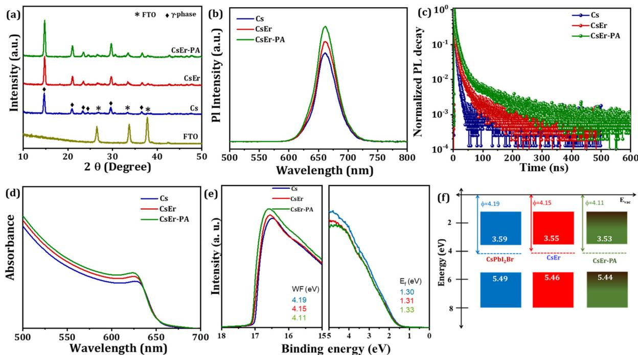
**Fig. 3** (a) XRD patterns, (b) photoluminescence, (c) time resolved photoluminescence, (d) UV-Vis spectra, (e) UPS analysis (f) energy-level diagram from UV-Vis and UPS measurements of the Cs, CsEr and CsEr-PA perovskite thin films.
