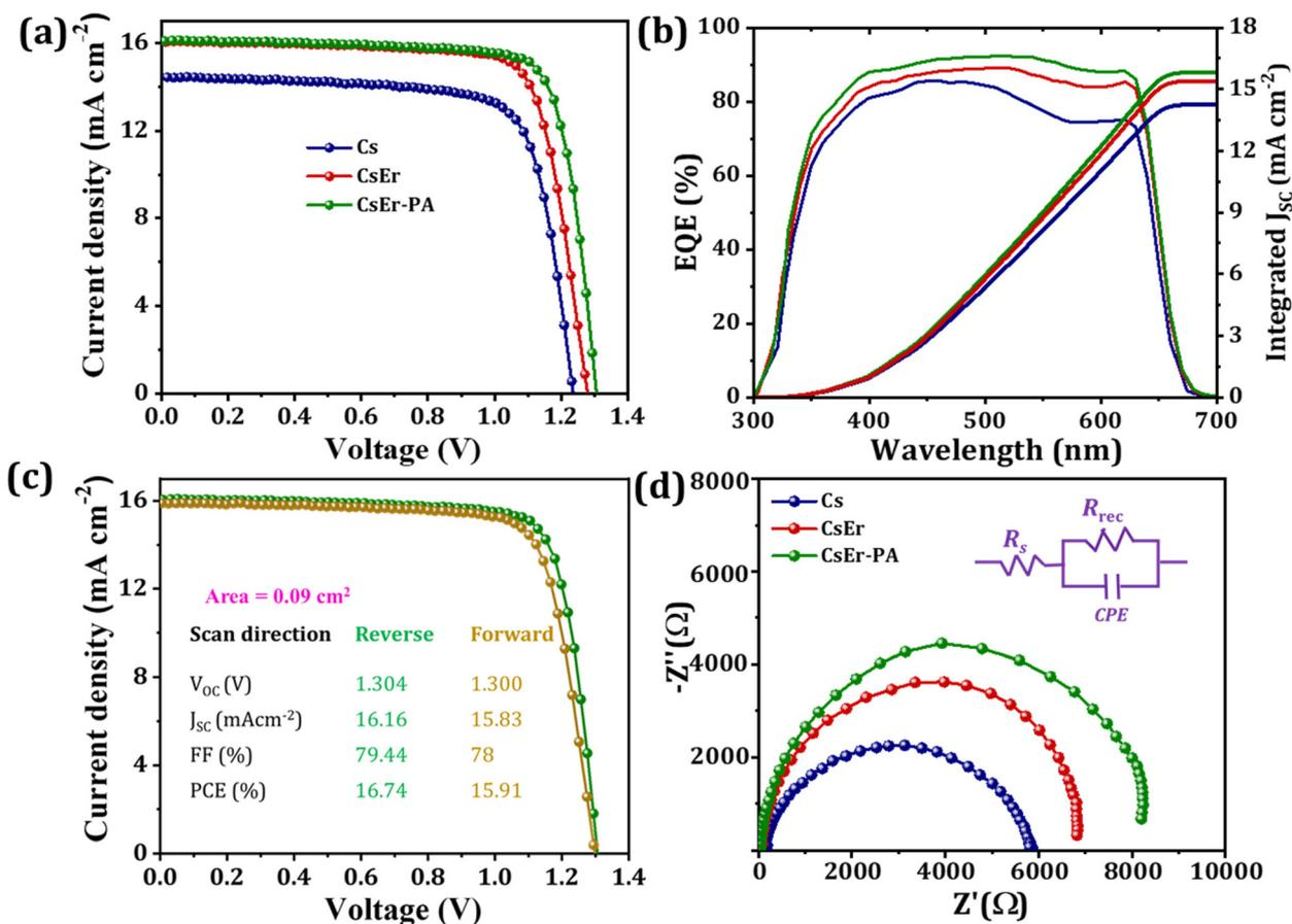
Fig. 4 (a)  $J$ – $V$  measurements, (b) external quantum efficiency (EQE) of Cs, CsEr and CsEr-PA-based perovskite devices, (c) hysteresis of the champion CsEr-PA-based device, (d) EIS analysis of the Cs, CsEr, CsEr-PA-based perovskite devices.
