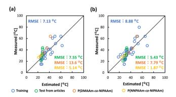
Fig. 5 The relationship between estimated  $T_{\rm CP}$ s from prediction model and measured values: (a) Compared by prediction model of eqn (1). (b) Compared by prediction model of eqn (2) with corrected coefficients.
