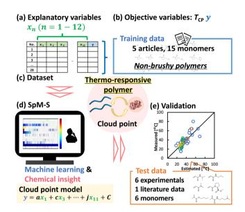
Fig. 1 Overview of this work: (a) 12 potential factors for  $T_{\rm CP}$  as explanatory variables. (b) Objective variables for training data of non-brushy polymers from 5 literature references. (c) Preparation of small dataset consisting of training data and explanatory variables. (d) SpM-S combining machine learning and chemical insight. (e) Validation of prediction model with test data.
