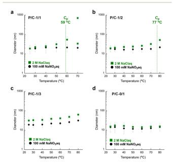
Fig. 6 Hydrodynamic diameter of (a) P/C-1/1, (b) P/C-1/2, (c) P/C-1/3, and (d) P/C-0/1 micelles and aggregates in water containing 100 mM NaNO $_3$  (black circles) or 2 M NaCl (green squares) at various temperatures (25, 30, 40, 50, 60, 70, and 80 °C): [polymer] = 1.0 mg mL $^{-1}$ .
