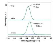
Fig. 12 C 1s (A), N 1s (B), O 1s (C) and Si 2p (D) XPS spectra of PMS before and after adsorbing TG. Following the completion of TG adsorption by PMS, specimens were obtained both before (PMS) and after adsorption (PMS-TG). XPS spectra analysis was conducted on each specimen, and the spectral information regarding the changes was processed using Origin software, including C, N, O and Si.
