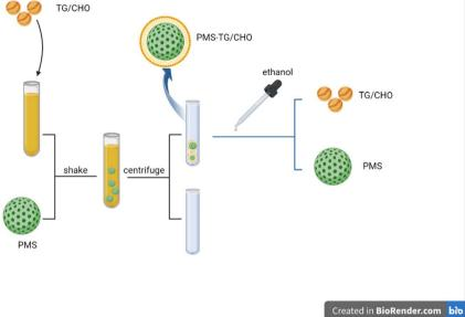
Fig. 1 Model diagram for CHO/TG adsorbed on PMS and separated from PMS. In brief, PMS was introduced into the CHO/TG solution to optimize the adsorption of CHO/TG onto PMS. Following centrifugation, the sediment was obtained, forming PMS-CHO/TG. Moreover, the addition of ethanol enabled the effective extraction and release of the adsorbed CHO/TG from PMS-CHO/TG.
