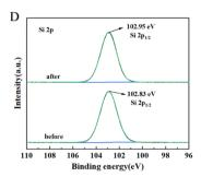
Fig. 11 C 1s (A), N 1s (B), O 1s (C) and Si 2p (D) XPS spectra of PMS before and after adsorbing CHO. Following the completion of CHO adsorption by PMS, specimens were obtained both before (PMS) and after adsorption (PMS-CHO). XPS spectra analysis was conducted on each specimen, and the spectral information regarding the changes was processed using Origin software, including C, N, O and Si.
