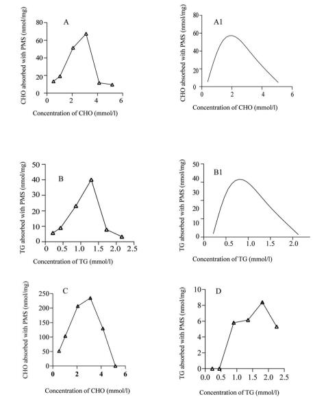
Fig. 3 The capacity of PMS for adsorbing CHO or TG at different concentrations. (A) The capacity of PMS for adsorbing CHO at different concentrations; (B) the capacity of PMS for adsorbing TG at different concentrations; (B) the capacity of PMS for adsorbing TG at different concentrations; (B) the capacity of polystyrene resin for adsorbing CHO at different concentrations; (D) the capacity of polystyrene resin for adsorbing TG at different concentrations.
