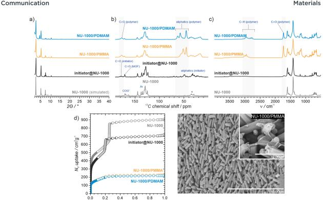
Fig. 3 Structural and morphological characterization of the initiator@NU-1000, NU-1000/polymer and pristine NU-1000 materials. (a) PXRD analysis; (b)  $^{13}$ C CP-MAS spectra; (c) DRIFT spectra; (d)  $^{13}$ C cp-MAS spectra; (c) DRIFT spectra; (d)  $^{13}$ C cp-MAS spectra; (e) SEM image of the **NU-1000/PMMA** hybrid.
