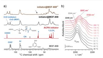
Fig. 2 Thermal decomposition of the ACPA initiator. (A)  $^{13}\text{C}$  CP-MAS spectra of MOF-808, pristine ACPA, and initiator@MOF-808 before and after thermal activation: the arrow indicates a signal sensitive to the initiator thermal activation. (B) VT-DRIFT spectra of initiator@MOF-808 (the C≡N vibration range) measured in the temperature range of 30-200 °C.
