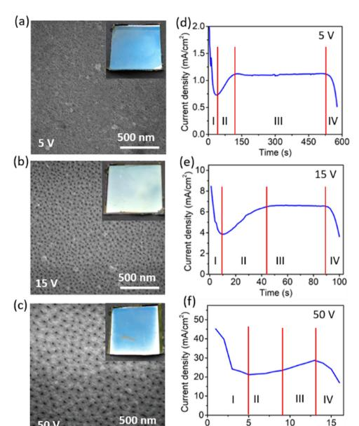
Fig. 2 FESEM images of the anodized nanoporous aluminium (AAO/AI) film at anodization voltages of (a) 5 V (b) 15 V and (c) 50 V. Inset images: photograph of the films, showing uniformity of the anodized film. Current density profile during anodization process at different applied anodization voltages of (d) 5 V (e) 15 V and (f) 50 V
