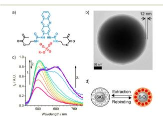
Fig. 2 a) Indicator crosslinker 1 presenting two polymerisable linkers and the bis-urea cleft able to complex phosphate anions; b) TEM image of a SiO<sub>2</sub>/MIP core-shell sensory particle M1 with shell thickness of 12 nm; c) emission spectra of the MIP sensory particles, M1, in chloroform upon addition of Fmoc-pY-OEt.TBA; d) scheme of the extraction and rebinding of the template molecule into the MIP shell.
