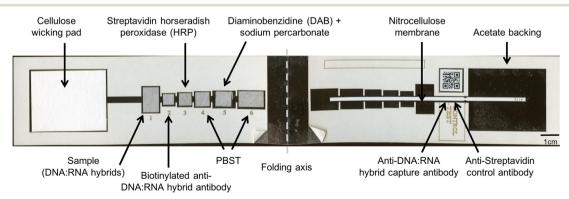
Fig. 1 Paper HPV DNA assay components. The paper assay includes a wicking pad, six glass fiber pads with lyophilized detection reagents to perform the hybrid-capture reaction, and a nitrocellulose membrane with capture antibodies spotted in designated test and control line zones, all placed atop an adhesive acetate backing. A QR code adjacent to the test and control lines facilitates use with low-cost readers. A 1 cm scale bar is shown.
