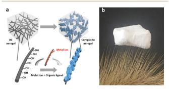
**Fig. 8** a) The fabrication process of BC@MOFs composite aerogels and b) photograph of the lightweight composite aerogels (reproduced from ref. 126 with permission from Elsevier Inc. copyright 2018).
