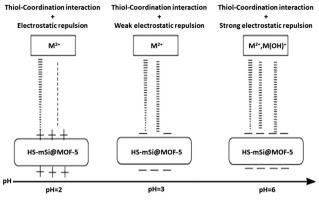
Fig. 13 A plausible mechanism of heavy metals adsorption over HSmSi@MOF-5 (reproduced from ref. 149 with permission from Elsevier Inc., copyright 2016).
