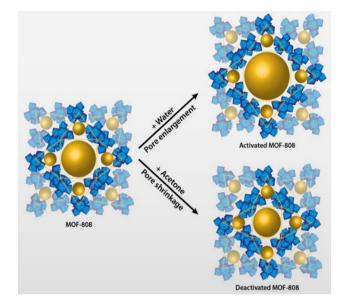
**Fig. 4** Hydractivation of MOF-808 showing pore expansion route with water after vacuum drying and hydradeactivation of pore shrinkage route with acetone after vacuum drying (reproduced from ref. 121 with permission from American Chemical Society, copyright 2018).
