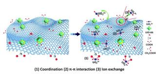
Fig. 9 Proposed mechanisms for the adsorption of  $U(v_1)$  onto GO-COOH/UiO-66 composites (reproduced from ref. 128 with permission from Royal Society of Chemistry, copyright 2017).
