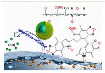
**Fig. 11** Cr(vi) reduction and immobilisation by the core-double-shell structured magnetic polydopamine@zeolitic imidazolate frameworks-8 microspheres (reproduced from ref. 130 with permission from American Chemical Society, copyright 2017).
