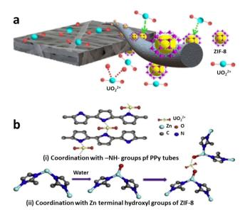
**Fig. 5** a) Schematic of the proposed adsorption mechanism of  $U(v_1)$  ions (reproduced from ref. 30 with permission from American Chemical Society, copyright 2018), and b) proposed mechanisms for the adsorption of  $U(v_1)$  onto PPy/ZIF-8 through i) MOF's organic linkers, and ii) MOF's metal nodes (reproduced from ref. 115 with permission from Elsevier Inc., copyright 2018).
