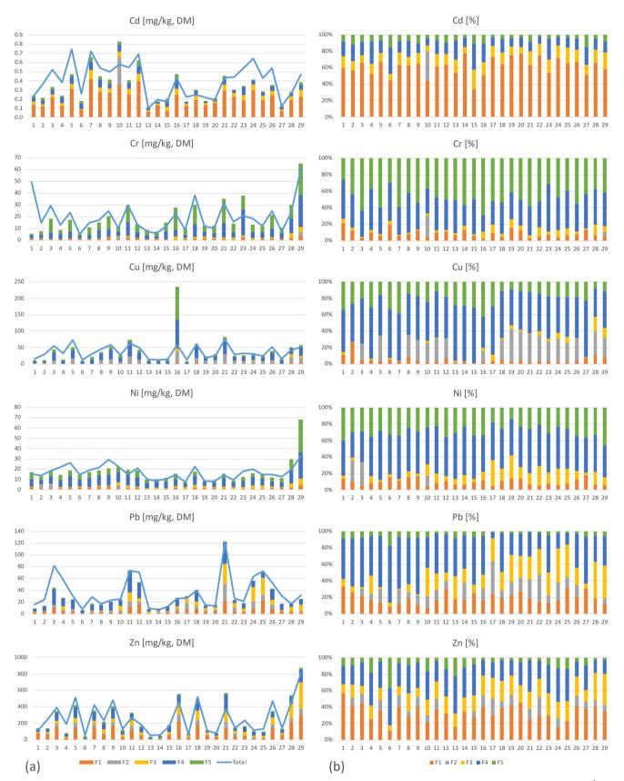
Fig. 4 Fractionation of Cd, Cr, Cu, Ni, Pb, and Zn for all sites (1–29). (a) The graphs to the left are reported as total concentrations (mg kg<sup>-1</sup>, DW), while those (b) to the right report the distribution between fractions (%).
