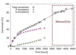
Fig. 6 Product formation at 20 °C with crystals encapsulated by glue. Product P is formed initially until ~20% conversion. Afterward, product Q is concurrently formed but at a slower rate. After, 2500 hours of reaction (~75% conversion) a phase change occurs from triclinic  $P\bar{1}$  to monoclinic C2/c, where the occupancies of products P and Q are about the same because the space group C2/c is centrosymmetric, and the structure refines with one unique product molecule in the asymmetric unit.
