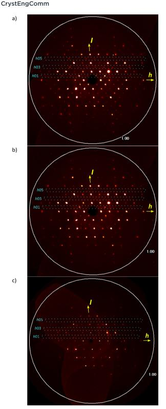
Fig. 8 Pseudo (h0l) precession images for (a) the room temperature reacted crystal at  $\sim$ 64% (just before transformation), and after the  $P\bar{1}$ to C2/c transformation at (b) ~79% and (c) ~89% conversion. The (h01), (h03), and (h05) reflections enclosed with dotted lines are allowed in the triclinic  $P\bar{1}$  space group (a) but are weaker in (b) and absent in (c) as required for C2/c.
