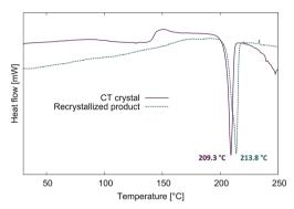
Fig. 11 DSC scans for a fresh CT crystal and a recrystallized crystal until their melting point. The CT crystal shows a reaction between  $100-150\,$  °C, and the melting peak is  $4.5\,$  °C lower than the recrystallized crystal.
