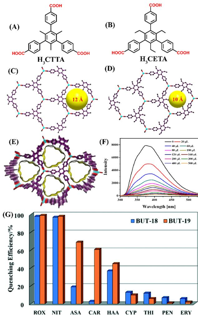
Fig. 3 The structure of organic linker (A) H<sub>3</sub>CTTA and (B) H<sub>3</sub>CETA. The framework structure of (C) BUT-18, (D) BUT-19, and (E) their 3D view of solid-state packing diagram. (F) The relative changes in fluorescence emission intensity for BUT-18 upon the addition of ROX in water. (G) The changes in emission intensity for BUT-18 and BUT-19 after the addition of different analytes. Reprinted with permission from ref. 61. Copyright 2019 Royal Society of Chemistry.
