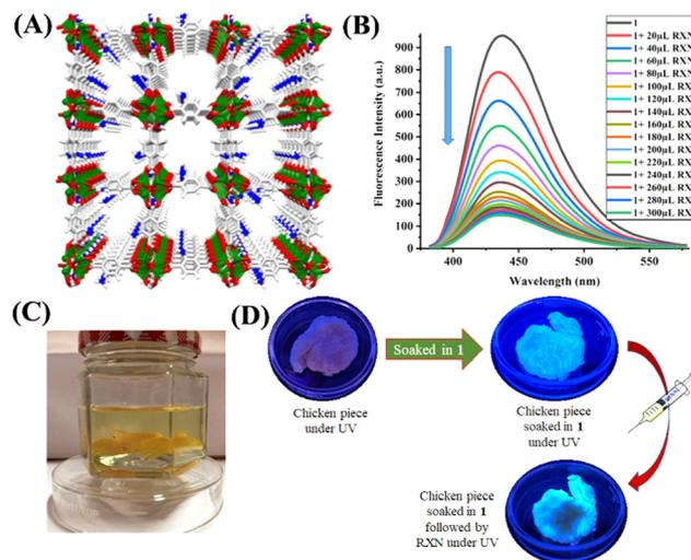
Fig. 8 (A) The 3D framework structure of luminescence Zn–MOF; (B) the changes in fluorescence emission spectra of Zn–MOF after adding increasing concentration of ROX (0–300  $\mu\text{L}$ ); (C) chicken piece immersed in the solution of ROX; (D) colorimetric response of the chicken piece soaked in Zn–MOF and followed by the addition of ROX. Reprinted with permission from ref. 75. Copyright 2022 American Chemical Society.
